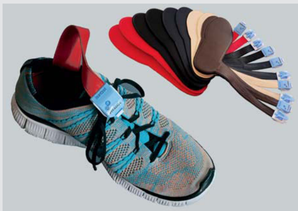
loadsol® insole in the shoe
