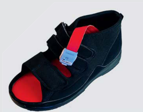
loadsol® with miniature electronics in a therapy shoe
