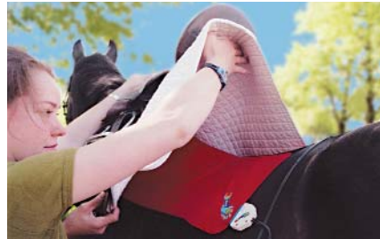
fixation of pliance horse sensor mat
