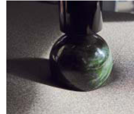
3D deformation of sensor mat
