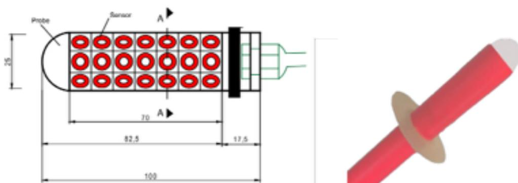
Figure 1. Instrumented vaginal probe
